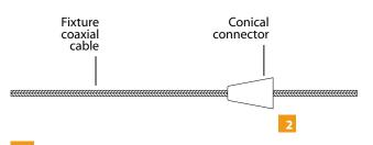
Insert the fixture coaxial cable through the conical connector
