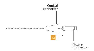
13 Slide the conical connector over the fixture connector.
